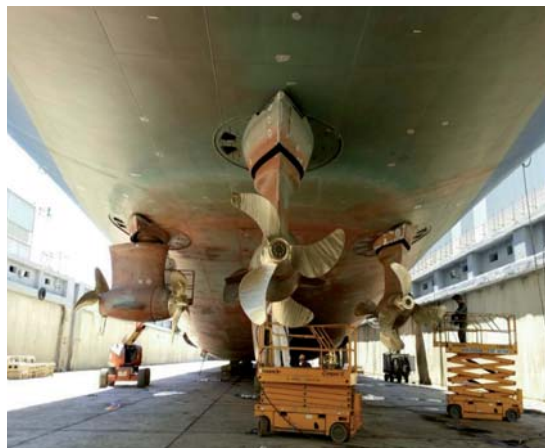
Fig. 14 – Propulsori Schottel Twin-Propeller STP 1515 FP. Fig. 14 – Schottel Twin Propellers STP 1515 FP.
