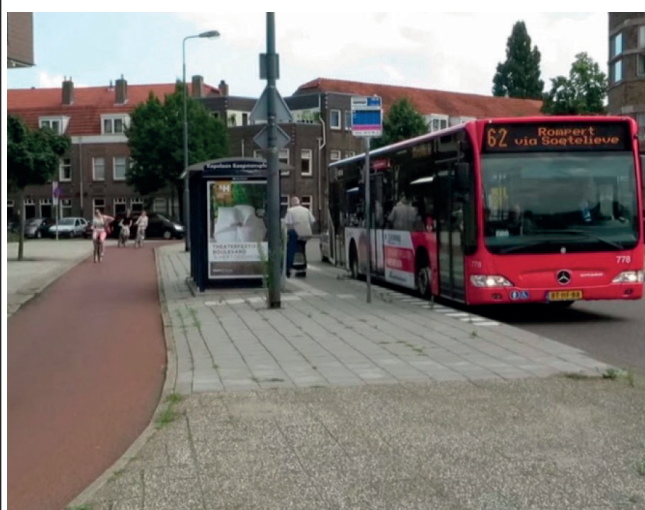
C - Pista ciclabile separata con isola pedonale - Lungo strada (Fonte: https://www.citylab.com/ ) C - Separate cycle path with pedestrian area - Along the road (Source: https://www.citylab.com/ )
