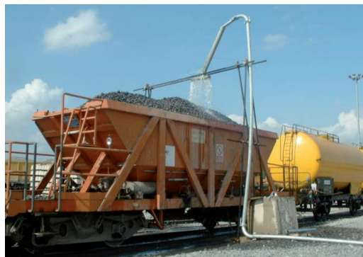
Fig. 16 - Cantiere CAR1. Impianto di lavaggio ballast. Construction yard CAR1. Ballast washing plant.
