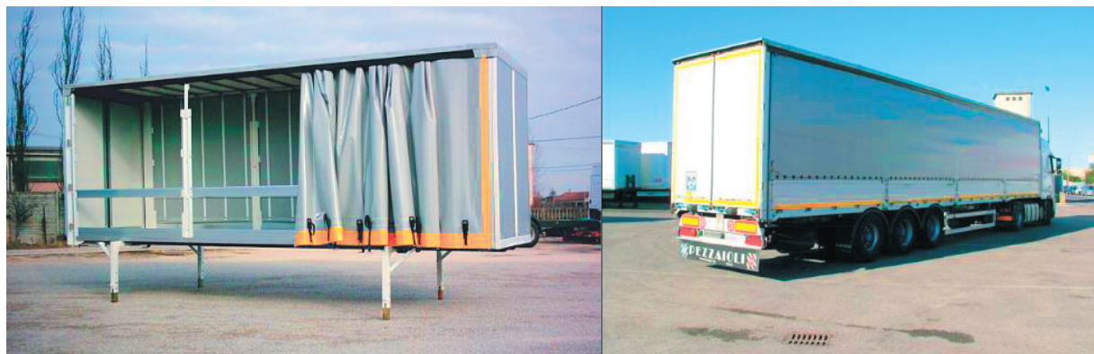
Figura 33 – Unità di trasporto intermodale alternative al container: cassa mobile (sinistra) e semirimorchio (destra). Figure 33 – Intermodal transport units alternative to the container: swap body (left) and semi-trailer (right).
