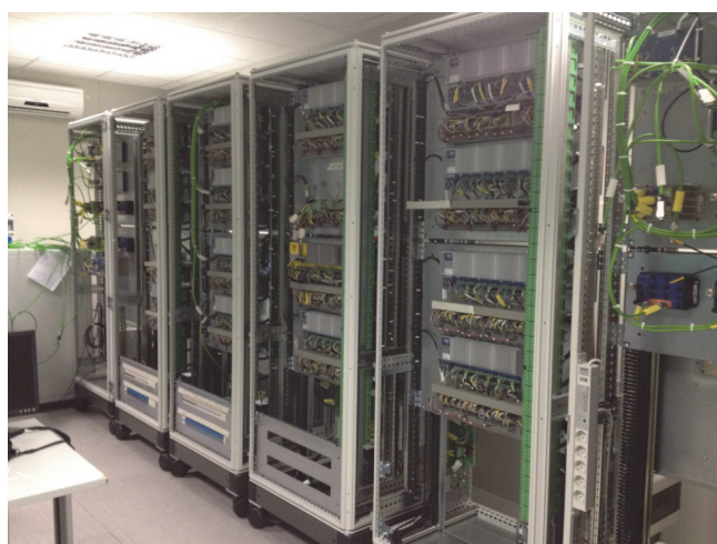
Fig. 5 - Rack con installati i dispositivi del TCMS. Fig. 5 - Rack with the TCMS devices installed.
