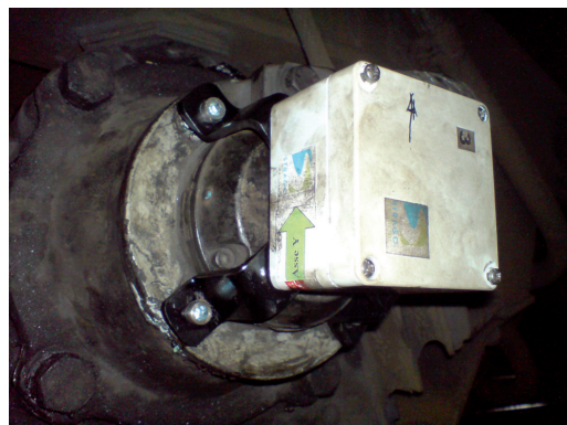
Fig. 3 - UF installata sul coperchio boccola. FU installed on the cover of the axle-bearing.
