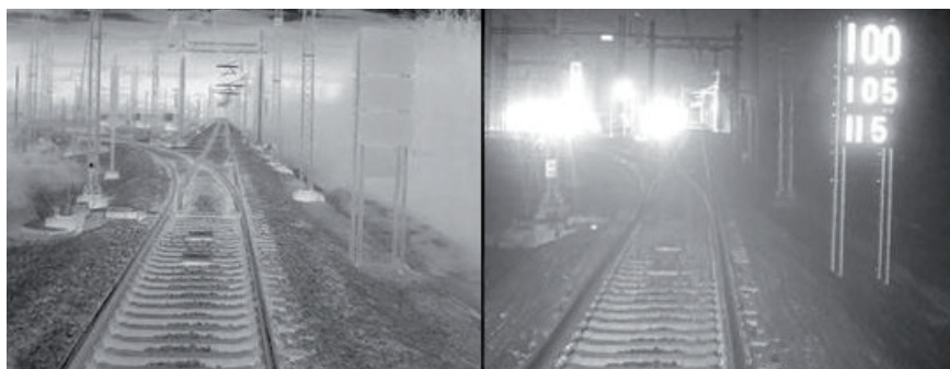
Figura 4 – A sinistra, immagine infrared; a destra immagine near-infrared. Figure 4 – On the left, infrared image; on the right, near-infrared image.
