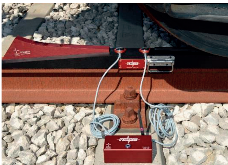
Figura 4 – Acquisition Board e Tablet con applicativo dedicato. Figure 4 – Acquisition Board and Tablet with a dedicated application.
