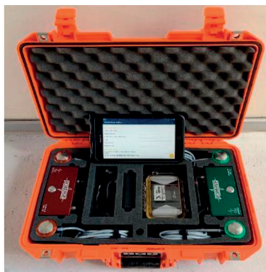
Figura 4 – Acquisition Board e Tablet con applicativo dedicato. Figure 4 – Acquisition Board and Tablet with a dedicated application.
